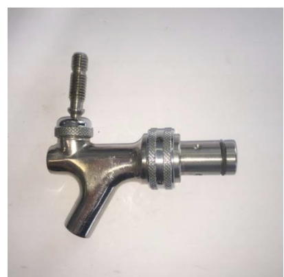
Step 8: Replace coupler gasket and fit shank. Fit coupler nut and gently tighten with C-spanner. Replace shank O-ring.
