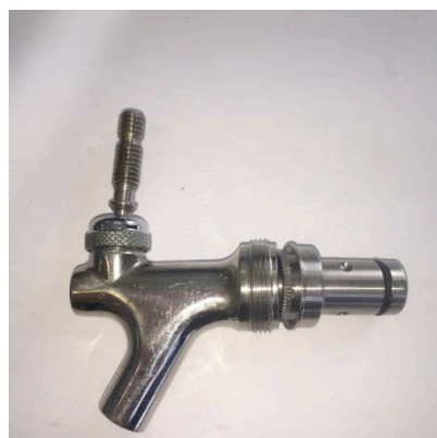
Step 8: Replace coupler gasket and fit shank. Fit coupler nut and gently tighten with C-spanner. Replace shank O-ring.
