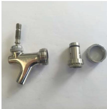
Step 1: remove coupler nut and shank (use of a C-spanner is recommended)
