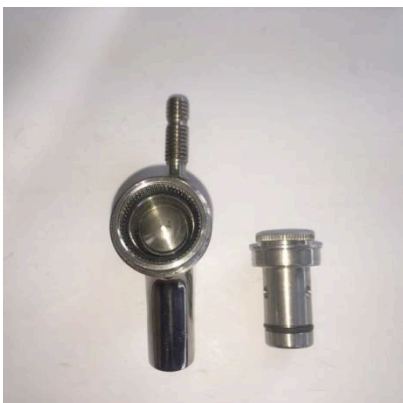
Step 8: Replace coupler gasket and fit shank. Fit coupler nut and gently tighten with C-spanner. Replace shank O-ring.
