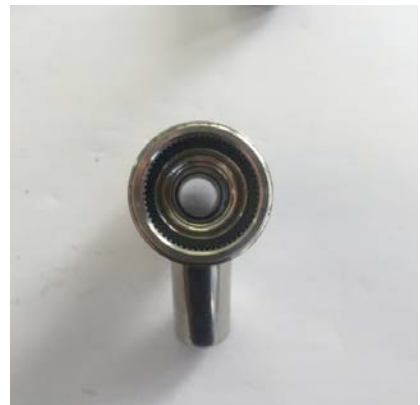
Step 5: Remove real coupler seal for tap shank from threaded end of tap.
