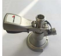
Line the probe "flats" in line with hinge pin entry. Push in hinge pin and fasten in place.. Push in hinge pin and fasten in place.
