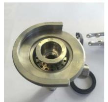
Re-Assembly : Replace the probe by inserting the threaded end of the probe into the body and slide in as shown below. Refit new keg seal.
