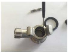
Step 3: There are 2 seals in the body of the keg coupler. Remove these and replace.
