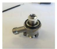
Replace the probe by inserting the threaded end of the probe into the body and slide in as shown below. Refit new keg seal.
