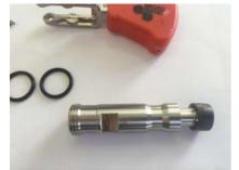
Step 3: Replace the probe seal as show below. Note that the seal has a split design on one side, the solid side of the seal face is to be installed so that it is visible.
