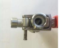
Step 1: Open the hinge pin by moving the retainer in line with the pin. Gently push out from the side with the hinged retainer as below.
