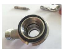
Step 5 : The last seal to change on the S-type keg coupler is the main gasket on the bottom of the coupler. The flat face of the seal is to be located against the body.
