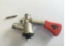
**Re-Assembly :** Insert probe into keg body (gasket end first). Have slot in line with hinge pin entry.
