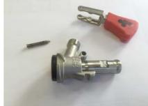
Step 2: Remove the hinge pin and then slide the handle backwards to remove from the probe. To remove the probe push from the side with the thick black seal until it can be removed from the handle side..
