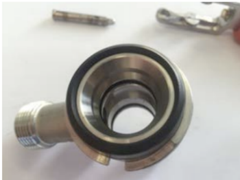
Step 4: The last seal to change on the D-type keg coupler is the main gasket on the bottom of the coupler. (see below) The flat face of the seal is to be located against the body.
