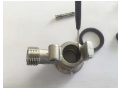
Step 2: Remove the hinge pin and then slide the handle backwards to remove from the probe. To remove the probe push from the side with the thick black seal until it can be removed from the handle..
