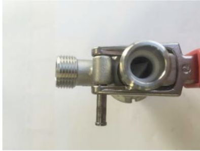
Step 1: Open the hinge pin by moving the retainer in line with the pin. Gently push out from the side with the hinged retainer as below.
