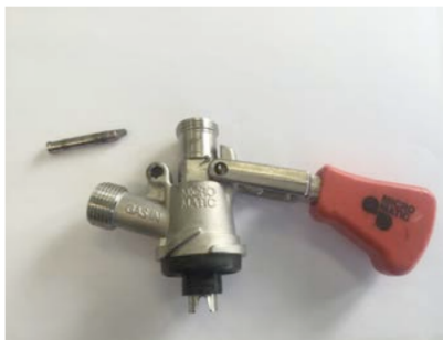
Re-Assembly : Insert probe into keg body (gasket end first). Have slot in line with hinge pin entry.
