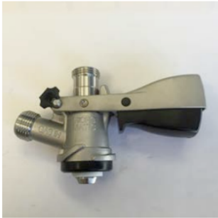
Step 1: Unclip hinge pin and remove pin, slide handle back to remove.
