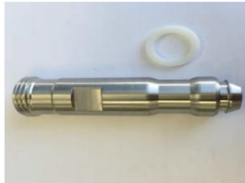
Re-Assembly : Insert probe into keg body (gasket end first). Have slot in line with hinge pin entry. Once probe is in the keg coupler body fit new white probe gasket.
