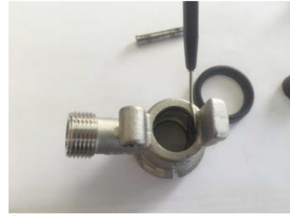
Step 3: There are 2 seals in the body of the keg coupler. Remove these and replace.
