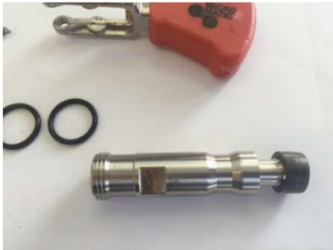
Step 3: Replace the probe seal as show below. Note that the seal has a split design on one side, the solid side of the seal face is to be installed so that it is visible.
