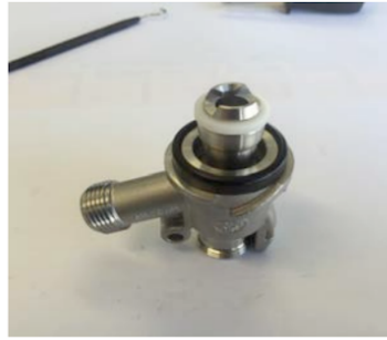
Step 2: Using a small flat head screwdriver or O-ring pick, remove white probe gasket to allow removal of probe. Push probe from gasket end out of the top of the keg coupler body
