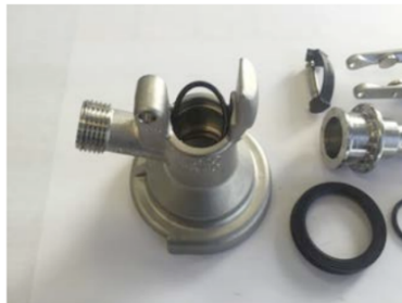
Step 4: There are 2 seals in the body of the keg coupler. Remove these and replace.
