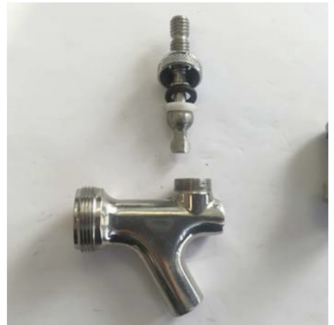
Step 2: loosen and remove handle lever assembly by rotating bonnet nut anti-clockwise. Pull lever away from tap.
