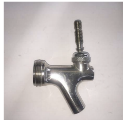
Step 7: Install white nylon friction with depression facing downwards. Install black friction gasket on top and screw bonnet nut clockwise. Tap should move fluidly with light pressure. Firm but free movement.
