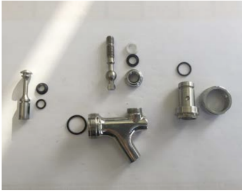
Standard seals requiring replacement.
