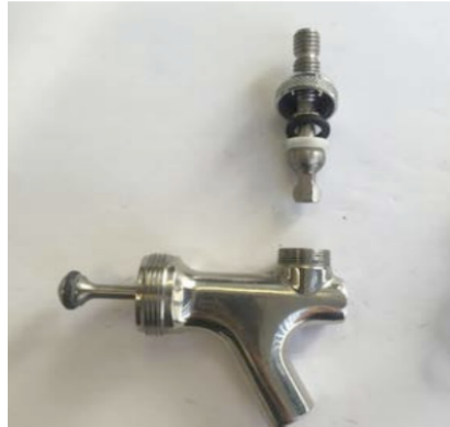
Re-assembly : Step 6: Push in piston into tap body.
